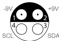
Probe's power supply pin assignment "cable view"
