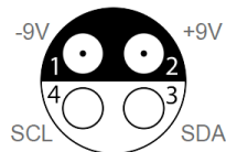
Probe's power supply pin assignment "cable view"
